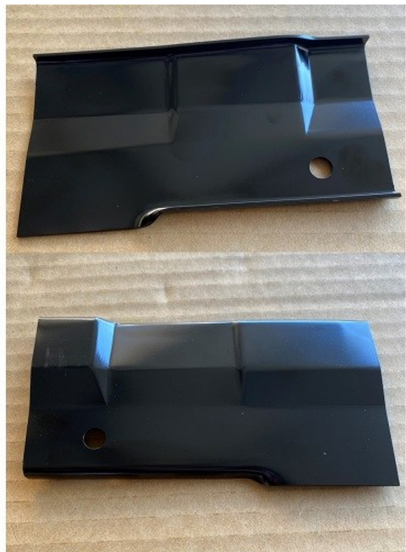
#208 XA-XC Upper Plenum Rect Reinforcing Plate RH
