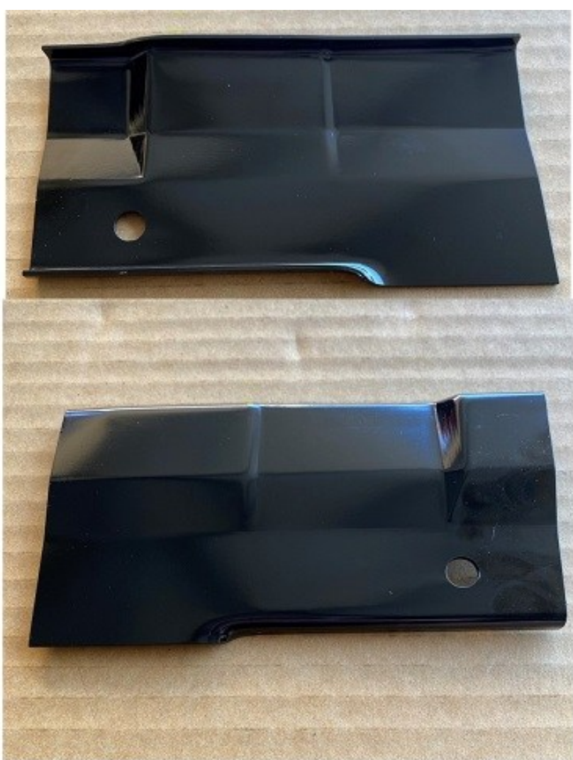
#207 XA-XC Upper Plenum Rect Reinforcing Plate LH
