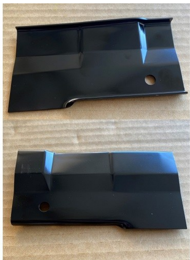
#208 XA-XC Upper Plenum Rect Reinforcing Plate RH
