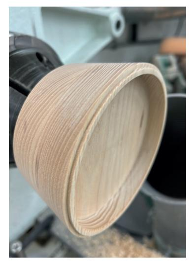
The lantern base parts were hand-turned on the wood lathe with the guidance of the workshop technician, as well as gaining experience using the 3-D form labs printer to make the clear resin base.
