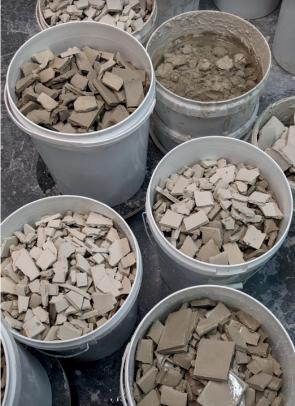
The Emerald Green and Crackle tiles are hand-extruded at the studio, followed by being cut and then fettled by hand. As there will always be waste it is important to reclaim the waste and re-use the reclaimed clay when extruding tiles again. This gives an overview of the whole process and how important all elements of the process are in production.
