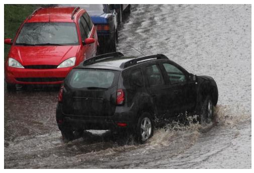
Vehicles stall out when water enters the exhaust pipe, usually when there is traffic and a car has to stop in high water to avoid hitting the person in front of them – even emergency vehicles and large trucks have this problem!
