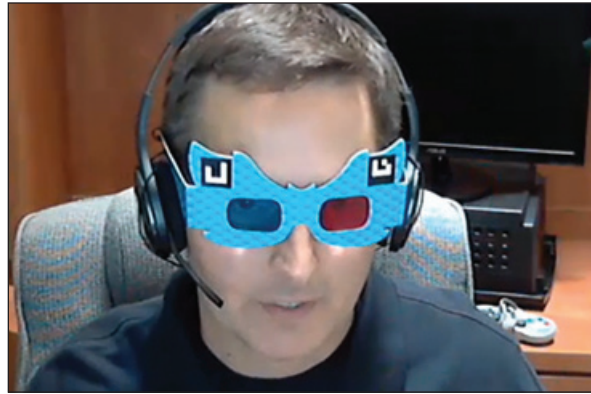
Figure 1. Barron Vision (Barron Associates, Inc) anaglyph glasses with tracking fiducials.
