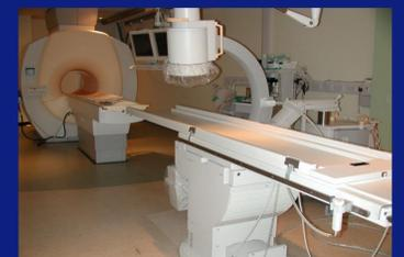
**Figure 5:** XMR system: a combined X-ray and MRI room where operating table slides into scanner.
