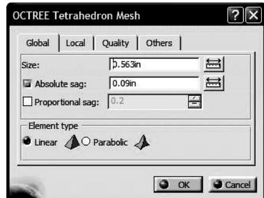
Notice that the type of the elements used (linear/parabolic) is also set in this box. Close the box by selecting **OK**.
