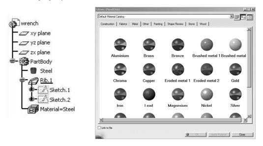
In order to inspect the values of the material properties assigned, double-click on **Steel** in the tree. It may take a minute before the database is searched. You will notice that the **Properties** box shown below opens. Choose the **Analysis** tab from this box, and the values will be displayed. Note that these values can be edited.
