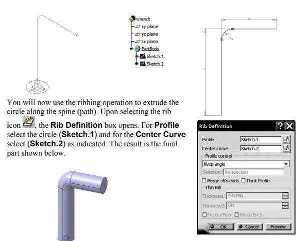
The next step is to apply material properties on the part created.
