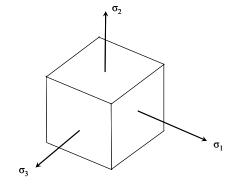
The principal stresses are postprocessed next. The principal directions are three mutually perpendicular directions along which only normal stresses act. These normal stresses are known as the principal stresses. The figure to the right displays the principal directions  $x_1$ ,  $x_2$ , and  $x_3$ , together with the principal directions  $\sigma_1$ ,  $\sigma_2$ , and  $\sigma_3$ . The standard convention in stress analysis is to label the stresses
