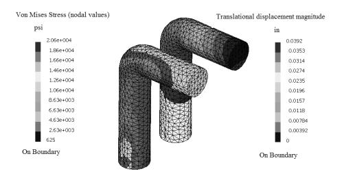
Before describing how the principal stresses are plotted, we like to elaborate on the significance of the von Mises stress plot.
