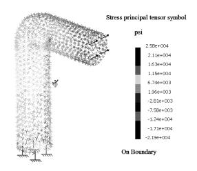
You can improve on the display of principal stresses by selecting a specific stress component to be plotted. To do so, double-click on the arrows on the screen which causes the **Image Edition**, shown to the right to open. Click on the **More** button to expand the window as shown below. Choose the **Component C11**. In CATIA, C11 represents  $\sigma_1$ , the largest principal stress.
