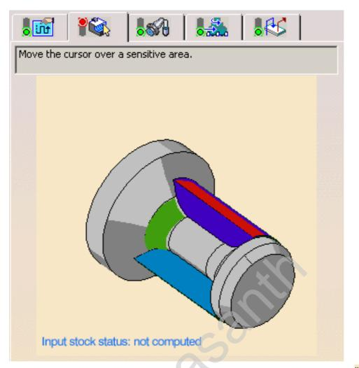
**6.** Select the **Update Input Stock** command by either clicking the icon **or** right-clicking the **Input stock status** field in the sensitive icon. The stock is computed and the corresponding sketch profile is displayed in the viewer.
