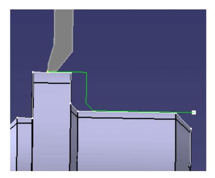
• **Radial part offset**: specifies a virtual displacement of the part profile in the radial axis direction.
