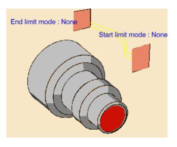
Local Information can be added on lines, arcs and curves if they are part of a finished profile. Click the red part in the icon then select the desired finish profile in the 3D window.
