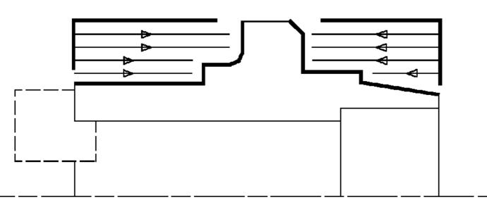
Orientation and Location settings determine the way the program closes the area to machine. The following options allow you to restrict the area to machine that is pre-defined by the stock and part. You may want to restrict this area due to the physical characteristics of the tool and the type of machining to be done.
