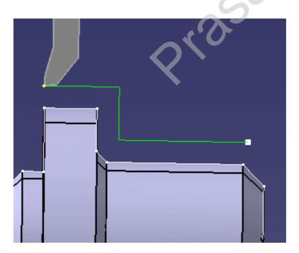
• Axial part offset: specifies a virtual displacement of the part profile along the spindle axis direction.
