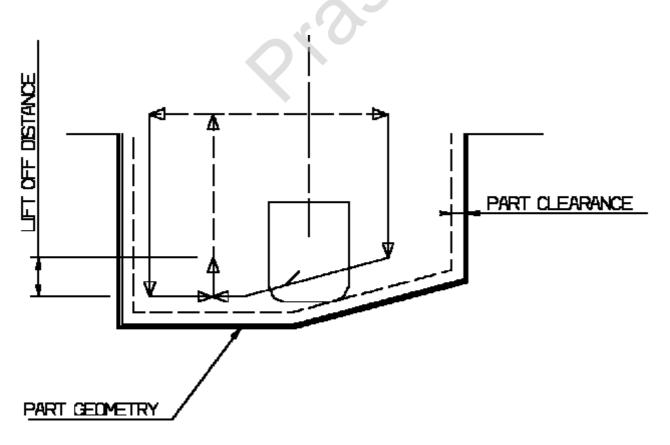
Lead-in, Lift-off and Attack for Recess Turning
