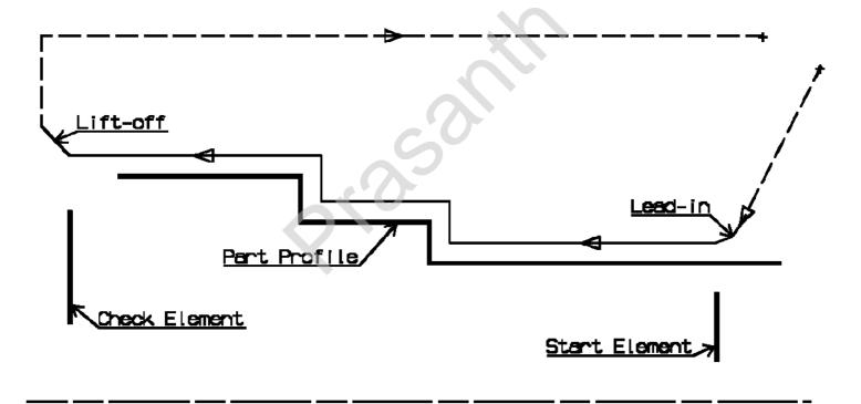
The figure above illustrates the use of start and end elements for Profile Finish Turning. Profile is machined from start element. Profile is extrapolated up to end element. Direct approach and radial-axial retract.
