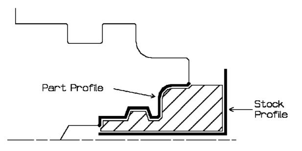
Frontal machining is proposed for face Rough Turning. In that case, the minimum and maximum diameters of the area to machine are determined by the stock profile dimensions.
