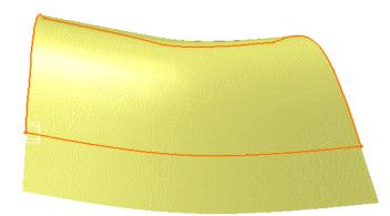
5. Select the Assemble result check box if you want the extrapolated surface to be assembled to the support surface.
