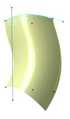
The figure below shows the result obtained when you include a linear spine element in the definition.
