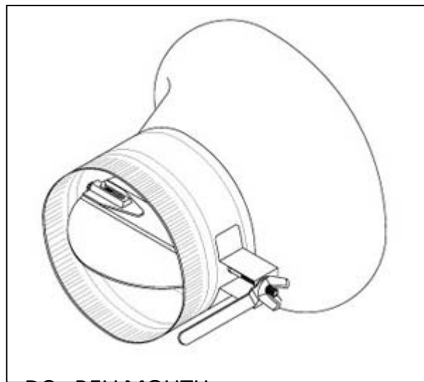
DC - BELLMOUTH EXTENDED BELLMOUTH With or Without Damper Available
