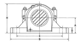
**Held and free:** Specify the appropriate stabilizing rings for a held unit; two required. Discard the enclosed stabilizing ring. For shaft diameter tolerances see page 359; for bearing information see page 97; for other seal speed limits see pages 347-350.
