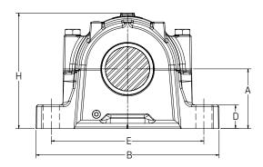
**Held and free:** Specify the appropriate stabilizing rings for a held unit; two required. Discard the enclosed stabilizing ring. For shaft diameter tolerances see page 359; for bearing information see page 96; for other seal speed limits see pages 347-350.
