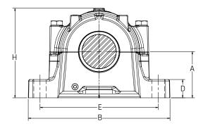
**Held:** Standard and standard option blocks come with a stabilizing ring. For toroidal bearings, the enclosed stabilizing ring must be used. For shaft diameter tolerances see page 359; for bearing information see page 192; for other seal speed limits see pages 347–350.
