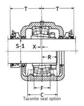
SAW 23500 Two-piece cast-iron housing Self-aligning / 23200 K series bearing Held or free bearing Oil or grease lubrication LOR triple ring seals Custom manufactured
