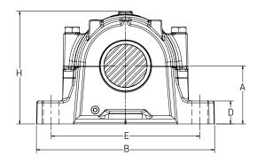
**Held and free:** Standard and standard option blocks come with an enclosed stabilizing ring. For a free unit, discard the enclosed stabilizing ring. For shaft diameter tolerances see page 359; for bearing information see page 164; for other seal speed limits see pages 347-350.
