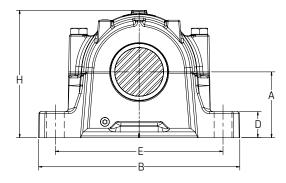
**Free:** Standard and standard option blocks come with a stabilizing ring. For toroidal bearings, the enclosed stabilizing ring must be used. For shaft diameter tolerances see page 359; for bearing information see page 192; for other seal speed limits see pages 347-350.
