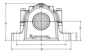
Held and free: Standard and standard option blocks come with an enclosed stabilizing ring. For a Free unit, discard the enclosed stabilizing ring.
