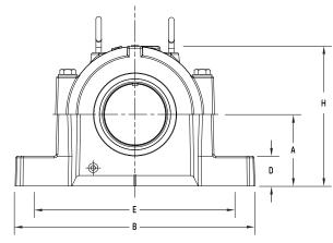
**Held and free:** Standard and standard option blocks come with an enclosed stabilizing ring. For a Free unit, discard the enclosed stabilizing ring. For shaft diameter tolerances see page 359; for bearing information see page 98; for other seal speed limits see pages 347-350.
