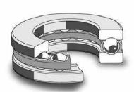
Single direction thrust ball bearing (data tables on page 112)
