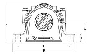
**Held and free:** Standard and standard option blocks come with an enclosed stabilizing ring. For a free unit, discard the enclosed stabilizing ring. For shaft diameter tolerances see page 351; for bearing information see page 164; for other seal speed limits see pages 339-342.
