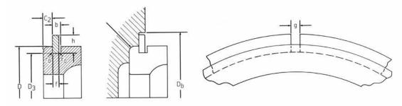
Snap ring and snap ring groove dimensions
