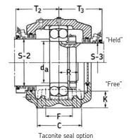
Two-piece cast-iron housing Self-aligning / 1300 series bearing Held or free bearing Oil or grease lubrication LER / LOR triple ring seals
