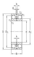
Double row Open, cylindrical and tapered bore Series: 2301 - 2320 M Size: 12 mm - 100 mm 0.4724 in - 3.9370 in
