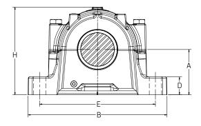
**Held and free:** Standard and standard option blocks come with an enclosed stabilizing ring. For a free unit, discard the enclosed stabilizing ring. For shaft diameter tolerances see page 359; for bearing information see page 162; for other seal speed limits see pages 347-350.
