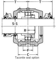
**Held and free:** Specify the appropriate stabilizing rings for a held unit; two required. Discard the enclosed stabilizing ring. For shaft diameter tolerances see page 359; for bearing information see page 97; for other seal speed limits see pages 347-350.
