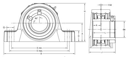
FSYE  $2^7/_{16}$  thru FSYE-4 supplied with single locking collar only FSYE  $4^7/_{16}$  thru FSYE- $4^{15}/_{16}$  supplied with double locking collar only
