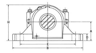
**Free:** Standard and standard option blocks come with a stabilizing ring. For toroidal bearings, the enclosed stabilizing ring must be used. For shaft diameter tolerances see page 359; for bearing information see page 193; for other seal speed limits see pages 347-350.
