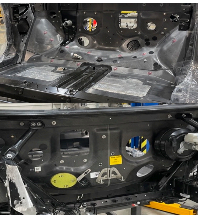
Advance integrated steel, Aluminum and carbon-fiber unified vehicle platform
