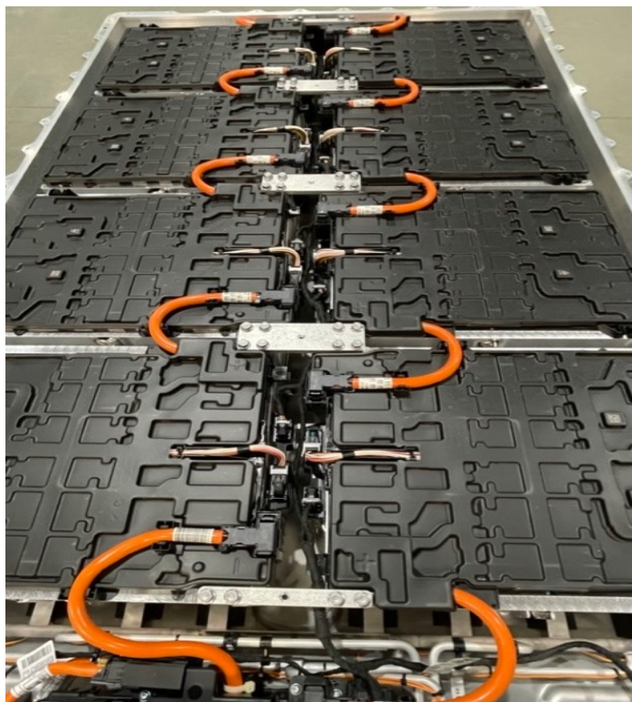
Prismatic high performance stable battery pack
