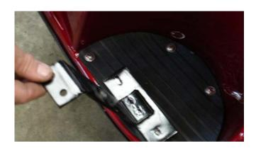
b. Position rear carrier rack on top of support brace, tighten those two bolts, and secure rack to vehicle with two bolts in holes at bottom of seat back.
