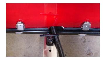
c. Then push T-handle back down securely to lock vehicle in preferred position.
