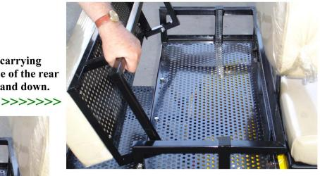
b. You now have a spacious, sturdy, rugged rear cargo carrier. (Simply reverse the procedure to return to the rear passenger seat mode.)
