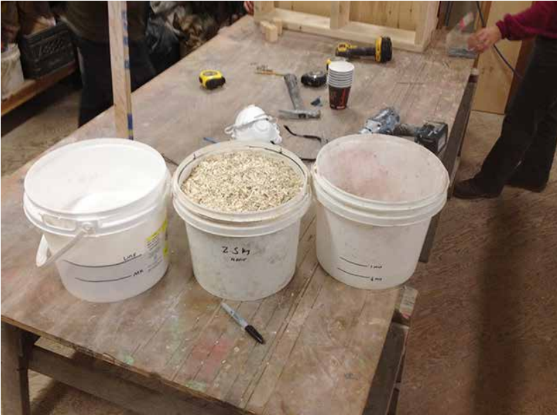
Buckets are marked so that the person making the mix can easily measure ingredients by volume and add them to the mixer.
