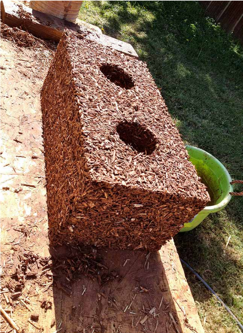
Two experimental forms of hempcrete are combined in this block cast using clay slip as the binder instead of lime.
