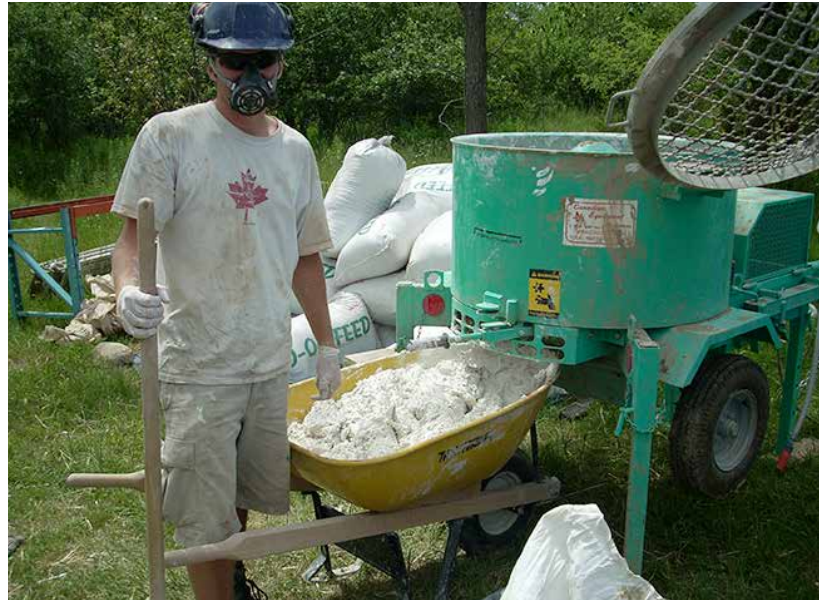
Specialty vertical shaft mixers are very good at mixing hempcrete, but may be harder to source than horizontal shaft versions.
