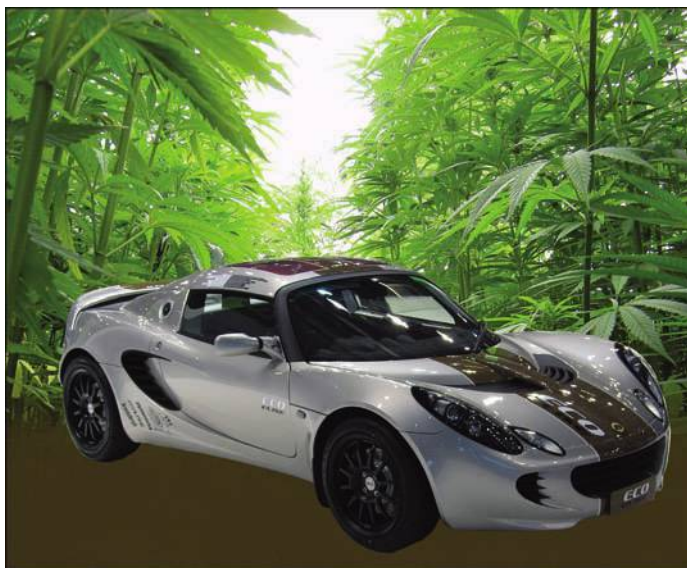
FIGURE 7.35 Lotus Eco Elise, body constructed of hemp plastic composite, introduced in 2008. Car photo by Stuart Chapman. (CC BY 2.0; hemp background added by B. Brookes.)
