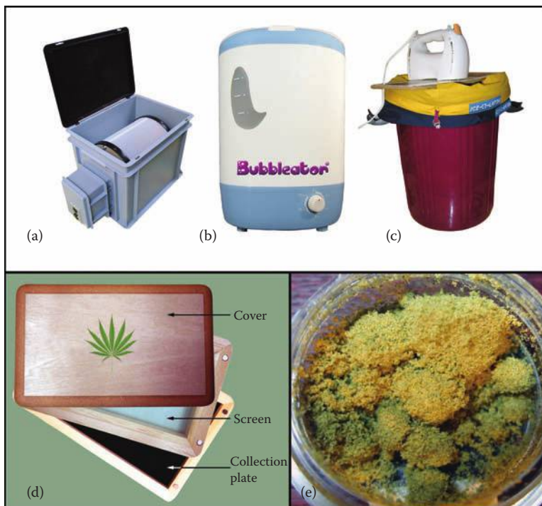
FIGURE 12.26 Top: recent commercially available extraction systems for preparation of purified, high-THC concentrates of secretory glands starting with herbal material (leaves and flowers). (a) The “Pollinator” is a dry sifting machine. Herbal material is placed in the revolving drum, which is perforated with 150 \mu\text{m} holes. Resin glands are expelled through the holes and collect in the box containing the drum. (b) The “Bubbleator” is constructed like a small washing machine. Frozen herbal material is placed, along with ice water, in a series of bags that are perforated with holes of decreasing size that permit the resin glands to be expelled. These in turn are placed in the device, which agitates the bags for a period, and then the separated resin glands are purified by additional sieving, and dried. This device takes advantage of the insolubility of the resin in water and the brittleness of the glands when frozen. (c) The “Ice-O-Lator” is a similar but simpler apparatus, in which an agitating device is placed on top of a bucket. Detailed operating instructions are available at various websites. These devices may be considered to be illegal drug paraphernalia in some countries. Photographs courtesy of Mila and Chimed Jansen of the Pollinator Company. Bottom: (d) “Kief box” (“pollen box”). This is a small box fitted with a fine screen through which bud is gently sifted, allowing mostly secretory trichome gland heads to fall through the screen onto a collection plate. (e) Cannabis resin powder. Photo by Mjpression (CC BY 3.0).
