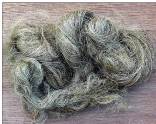
FIGURE 7.19 Raw cleaned hemp fiber (the thread-like materials are bundles of primary hemp fibers; cf. Figure 7.14c ). Photo by Rasbak (CC BY 3.0).
