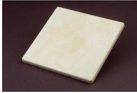
FIGURE 7.33 Hemp “ceramic tile.” Photo by E. Small, tile furnished by Kenex Ltd., Pain Court, Ontario.
