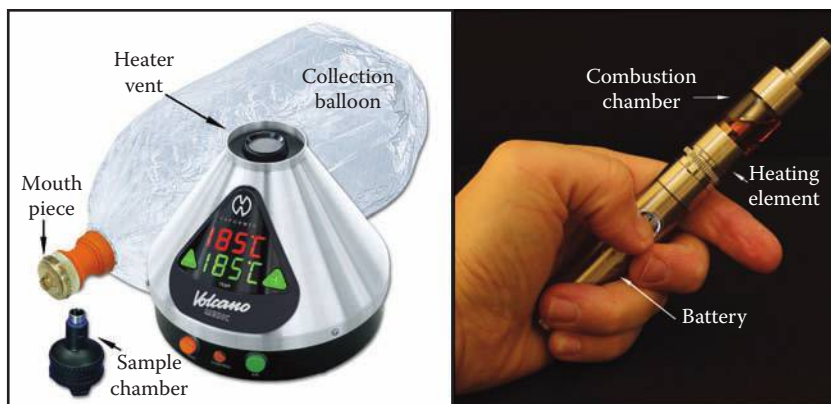
FIGURE 13.11 Vaporizers. Left: The Volcano vaporizer system for volatilizing the resin of C. sativa . This is the most extensively studied vaporizer available and has been used extensively in medical studies. A receptacle (“sample chamber”) containing ground material is placed in the “heater vent” at the apex of the pyramid-like apparatus, where heat volatilizes the active components of the resin. The resulting gases are collected in the balloon, and the contents of this are inhaled. Such devices can greatly reduce the number of inhaled dangerous components that are present in marijuana (performance of the Volcano vaporizer was evaluated by Gieringer et al. 2004). Photo by Storz & Bickel (CC BY 3.0). Right: A portable electronic (“vape pen”) vaporizer. Photo by Jonny Williams/www.ecigclick.co.uk (CC BY SA 2.0).
