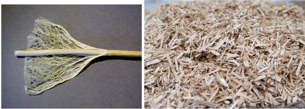
FIGURE 6.1: Indication of the hemp stem and fibers (left) [?] and hemp shivs (right)[?]
