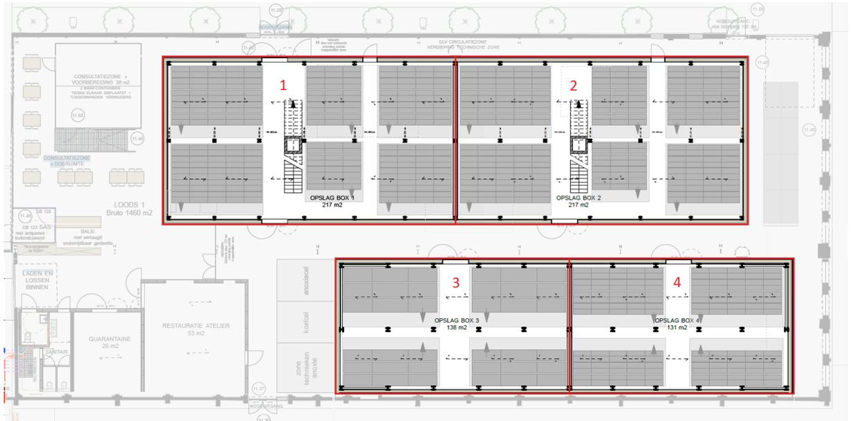
FIGURE 3.4: Top view of hempcrete boxes ground level
