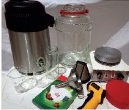
**1. Equipment required: still or rice cooker; assorted glassware; funnels & filters; hotplate with variable temperature control; and laser thermometer.**
