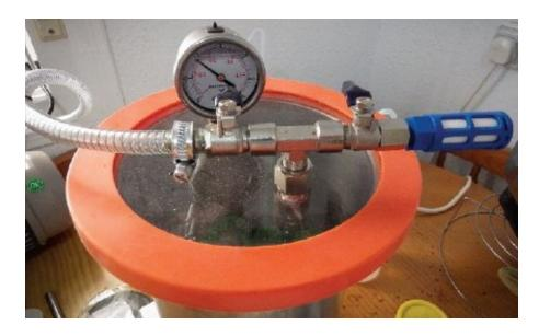
22. By using a vacuum chamber you can remove all the traces of butane to create 'shatter.'
