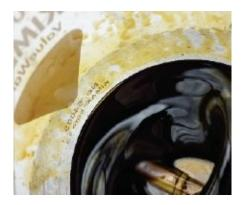
21. You can control the speed of the magnetic stirrer bar. Keeping your oil moving helps to avoid 'hotspots.'
