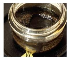
6. Once most of the solvent is evaporated pour the solution into a glass container and put it in a coffee warmer for the final evaporation process.
