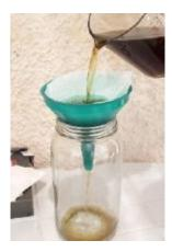
12. Remove the finer particles by filtering through unbleached fine coffee filters.
