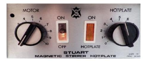
19. For the final stage, transfer the oil to a hotplate with variable temperature control. The authors use a magnetic hotplate stirrer. This useful device keeps your oil moving.
