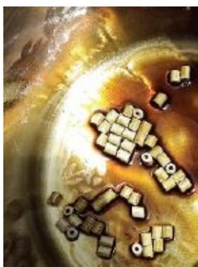
**18. For this batch the authors used a still. The ceramic rings seen here aid the evaporation process.**
