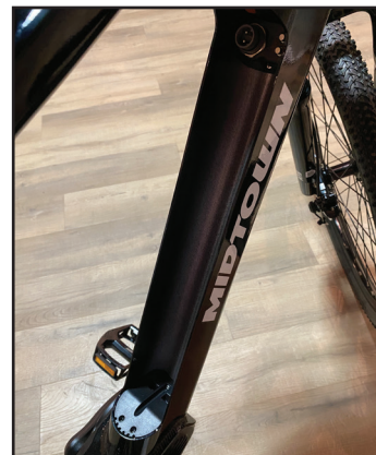
Battery removed from the frame
