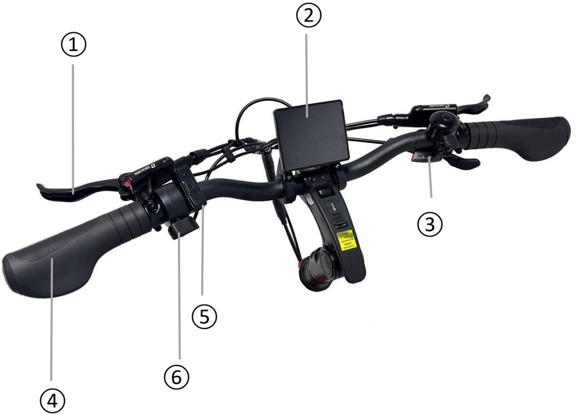
1. Left Brake Lever for front brake
