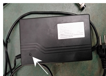
Green light indicates charging finished
