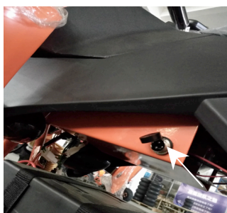
Insert charger output terminal to the charging port
