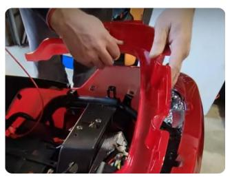
Now is also a perfect time to double check that all the electrical connections on your scooter are secure. Reconnect any separated connection or tighten any loose ones. Please note there will be extra connections on the controller, not used in the function of your scooter.
