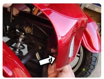
Next align the side holes on the hood with the side mounting brackets. Please note the hood may have warped during shipping, if the holes do not align *carefully* bend the hood so they do. Once aligned insert bolts (e) on each side and then tighten them and the front bolt.
