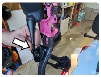
Secure the mirrors into place with the bolts (f) on the outside, and the nuts (n) on the inside.
