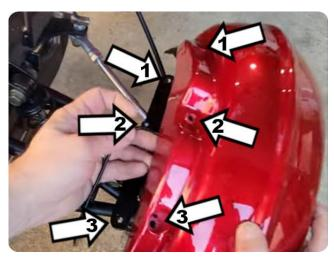
Please make sure the cable for the integrated LED lights is on the outside of the bracket, not between the bracket and tire.
