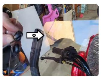
Secure the windscreen to the 2 mounts below the windshield brackets with the shiny aluminum washers (q) and hex bolts (k).
