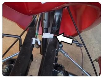
Attach each fender with bolts (h) in each of the 3 holes. Connect the connector from the fender lights to one of the 3 connectors on the front end.
