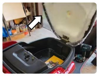
With it now unlatched you can lift the seat cushion forward and remove the 4 bolts holding the underseat tray in position. Carefully set the seat aside as it will still be attached via the cable on the seat latch. You can now access the piece of trim that also needs to be removed, remove all the screws holding it in place.
