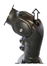
Insert the handlebar stem over top of the steerer tube and align straight forward. (perpendicular to the front wheel) Then tighten the bolt that was concealed by the plug into the hole that held the protective cap, as well as the 2 bolts on the front of the stem.
