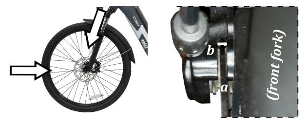
Once in place, snug the capped nut until the lever on the brake side requires enough pressure to close that it leaves an imprint on your hand when closing.
