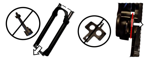
Steadying the wheel vertically, carefully lift the front forks over the axle, slot the brake disc(a) in between the brake pads of the brake caliper(b), and lower the forks squarely onto the axle.
