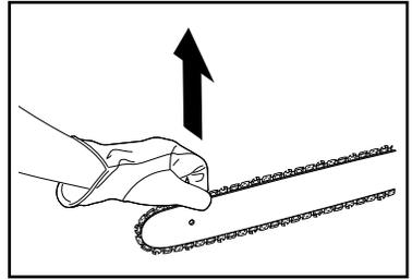
**NOTE:** If the chain is too tight, it will not rotate. Loosen the chain cover lock nuts slightly and turn the chain adjustment screw 1/4 turn counterclockwise. Lift the tip of the guide bar up and retighten the chain cover lock nuts. Ensure that the chain will rotate without binding.
