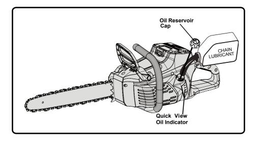
**NOTE:** Chain saw comes from the factory with no bar and chain oil added. The level should also be checked after every 20 minutes of use and refilled as needed.
