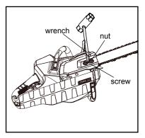
**NOTE:** During normal saw operation, the temperature of the chain increases. The drive links of a correctly tensioned warm chain will hang approximately 1/16 in. (1,58 mm) out of the bar groove.
