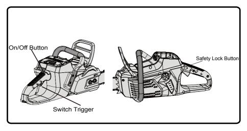
NOTE: It is normal for the chain to coast to a stop once the trigger switch is released.
