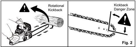
**2.** Do not overreach and do not cut above shoulder height. This helps prevent unintended tip contact and enables better control of the chain saw in unexpected situations.
