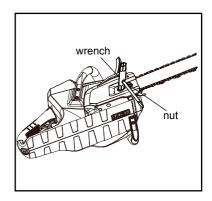
• Rotate the chain adjustment screw clockwise to increase the chain tension and rotate counterclockwise to decrease the chain tension.
