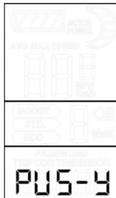
Button walk assist enable setting
