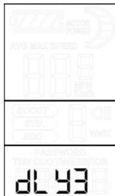
Battery delay time setting
