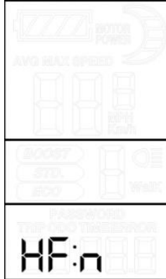
Throttle level enable setting
