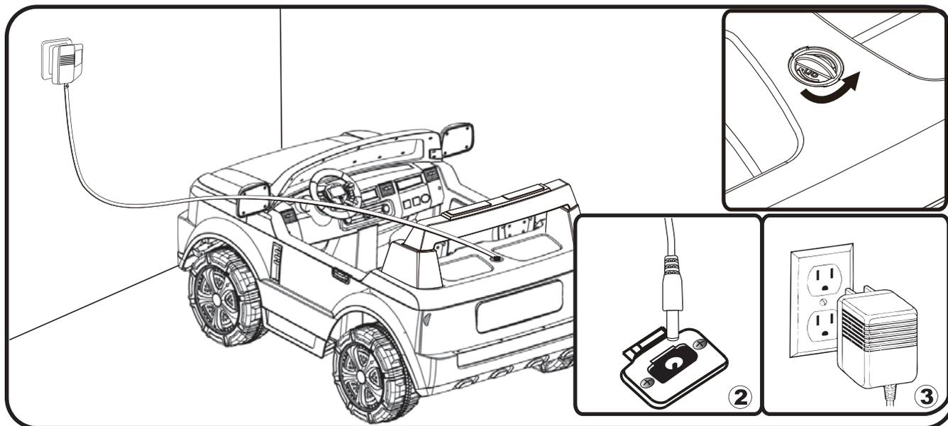
1. Open the cover of the socket (the socket is under the rear light bar)
