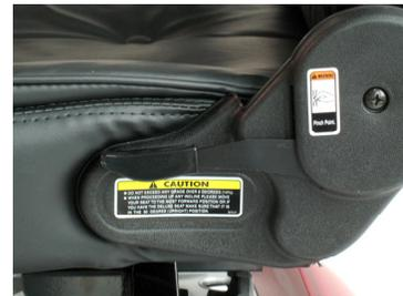
**Slide** - To move closer or farther away from the tiller, push down on the black lever handle located under the center of the seat and slide to your desired position.
