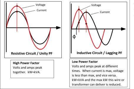
Power factor correction equipment restores the capacity by pushing the two waves closer together.
