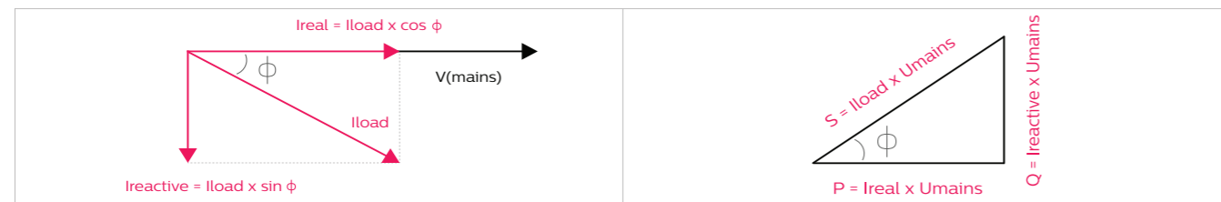
Figure 5: A: current decomposition, B: power triangle
