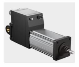
Upgrade to an actuator with a <u>brushless</u>, DC motor which is controlled by an <u>onboard</u> motor drive. **Brushless motors require no maintenance.** Onboard drives are managed by controllers, without the need for a third amplifier box.
