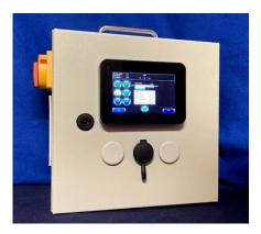
Improve your controller. EDGE controllers offer a color touchscreen HMI for operator interface, connect to all industrial networks, can control remotely via a wireless network, operates both electro-mechanical and hydraulic actuators.
