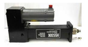
Upgrade your obsolete, brushed DC motor which is controlled by a remote motor drive. **High thrust actuators, rated in 2,000, 4,000, and 6,500 ft-lbs. of thrust utilize DC brushed motors.** The brushes require maintenance. The manufacturers of the motors are gradually obsoleting the motors and therefore the actuators will also become obsolete. The linear thrust is produced by a **ball-screw actuator** which under-performs as the thrust increases.
