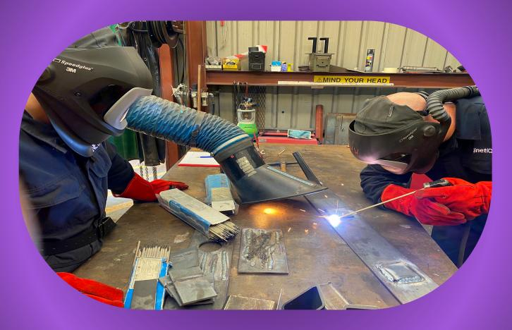
An introduction to the MMA welding process covering: How to set up the equipment, selecting the correct consumables and basic techniques for a range of applications and metals.
