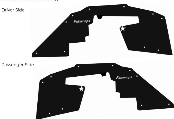
The following diagram indicates the position for each clip type: 8mm x 20 and 7mm x 2  $\frac{1}{24}$
