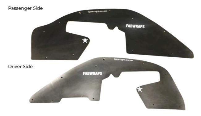
Clip Tip: Pull the 8mm clip apart, place the back piece into the guard, fit guard to the car and then push the clip top into place to secure.
