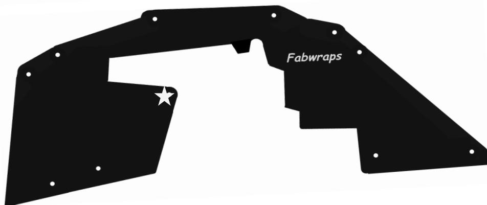
*Clip Tip: Pull the 8mm clip apart, place the back piece into the guard, fit guard to the car and then push the clip top into place to secure.*
