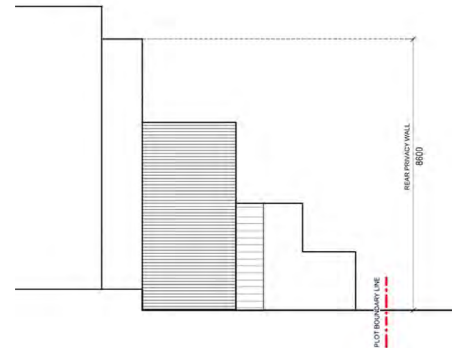
Figure 14a: Right Elevation (Canal side) showing boundary wall for 4.2 / Aseel Applicable for Inner Canal Villas (*Note: Rear Privacy Wall length will vary as per plot size)
