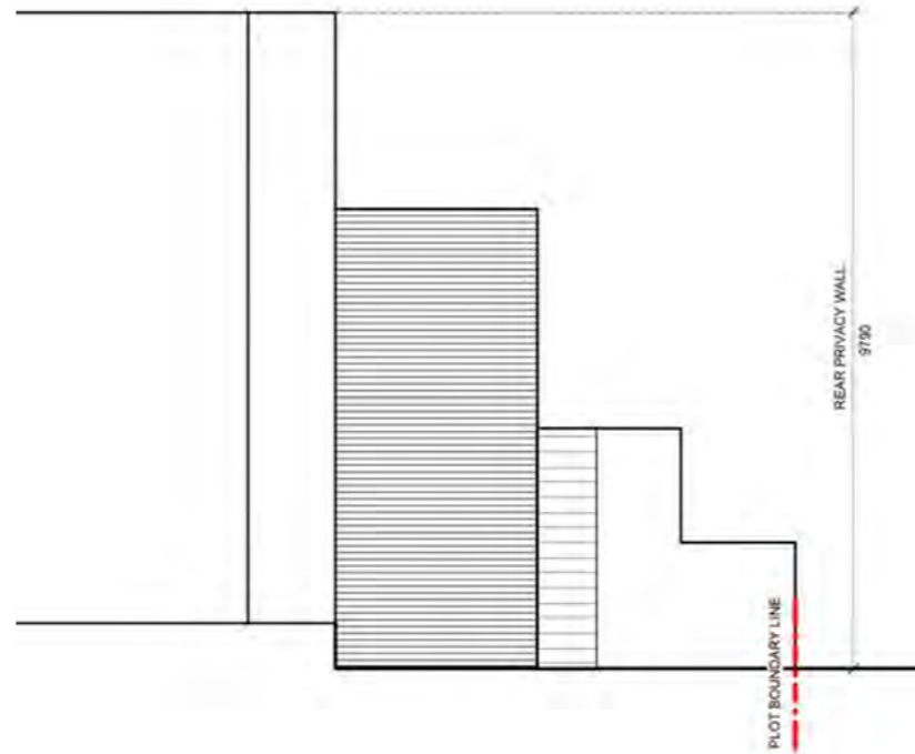
Figure 14: Right Elevation (Canal side) showing boundary wall for 4.2 / Aseel Applicable for Outer Canal Villas (*Note: Rear Privacy Wall length will vary as per plot size)
