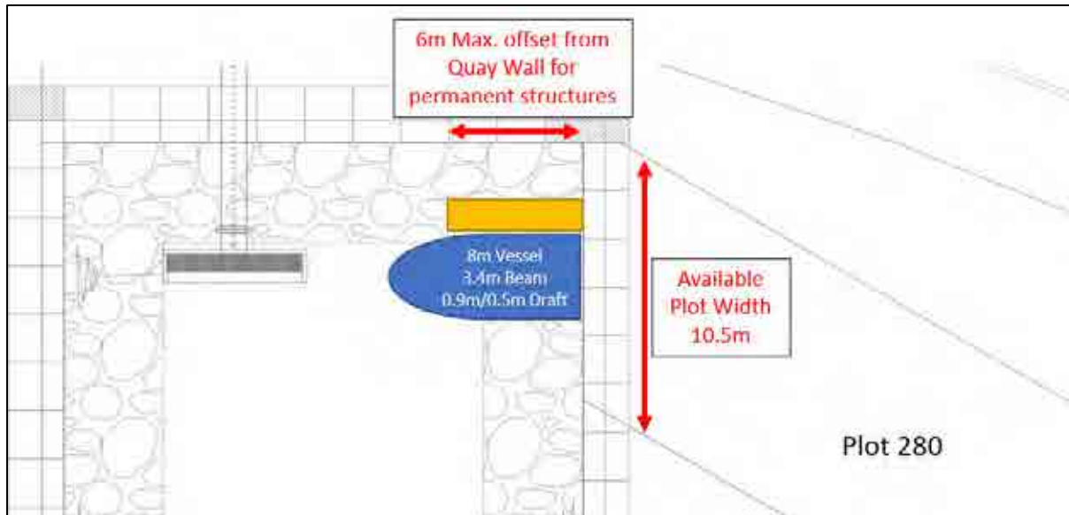
Figure 3-13 – Proposed Parallel Mooring Arrangement for Plot 280
