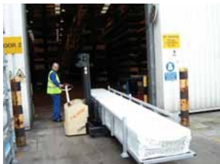
Easy switch over from lengthwise to crosswise driving via push button in the drawbar head.
