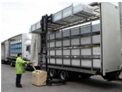
Easy switch over from lengthwise to crosswise driving via push button in the drawbar head.
