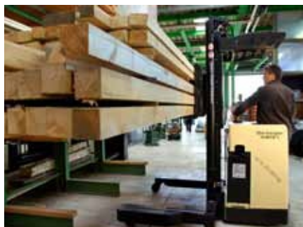
Transport of long and bulky loads through narrow aisles and doors.
