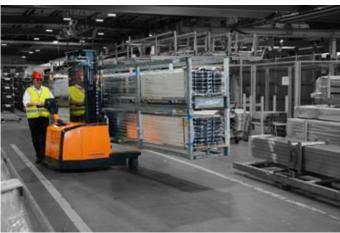
Four-way chassis for easy switch over from lengthwise to crosswise driving.
