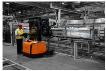
The robust pantograph is lifting the long load.
