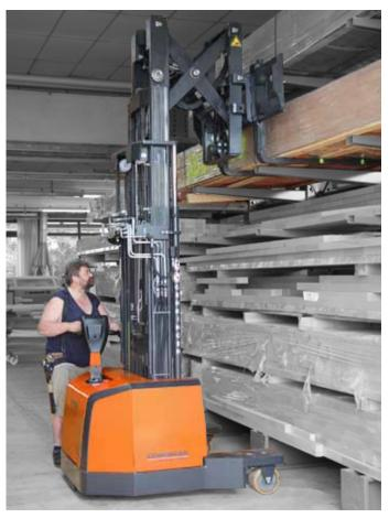
Ideal positioning in front of racks due to pantograph.
