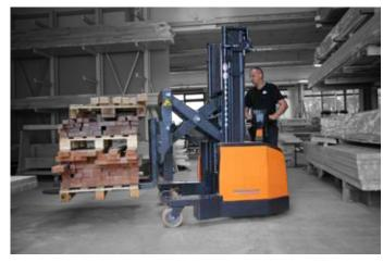
Comfortable lifting of pallets from the floor.
