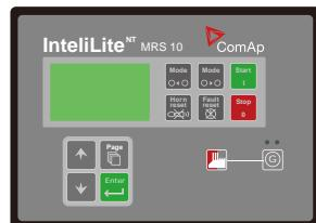
Support engine and alternator monitoring, measurement and protection. This is long-running and back-up unit to integrate the best way to control. support Modbus standard, modem, RS232, RS485, USB and internet.
