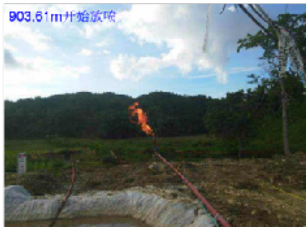
Gas discharging from a depth of 903.61m
