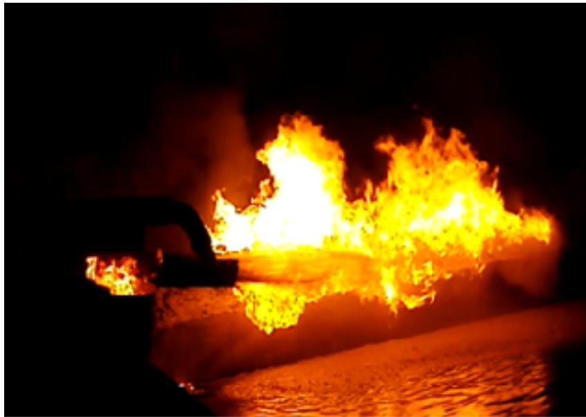
Oil & Gas discharging from well during Polyard-3 Well testing
