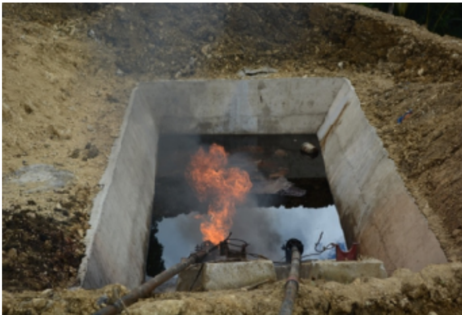
Oil & Gas discharging from well during DST of Polyard-1 Well.
