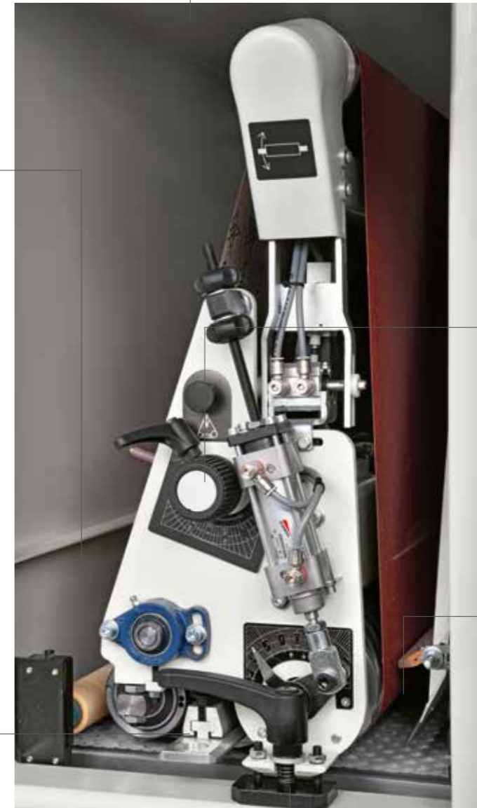
Semi-stiff flat pad for veneered panels sanding
