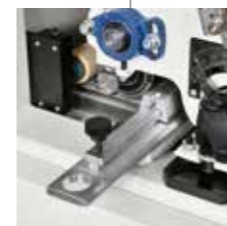
Semi-stiff flat pad for veneered panels sanding
