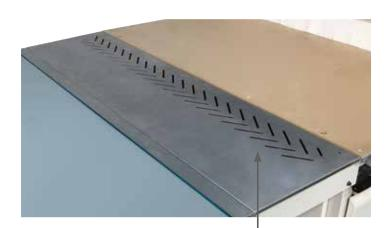
**Clean work environment** with the chips conveying device positioned between the work table and the unloading belt.
