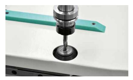
**Tool length detection device**Positioned on the machine base side, it allows to automatically detect the length of the tool.
