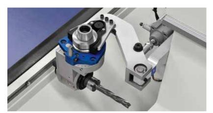
One position "Pick-up" tool changer with pneumatic positioning fitted on the mobile cross beam.
