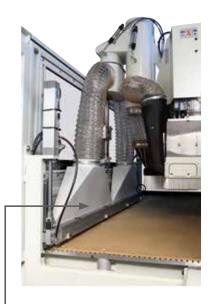
**No dust** with the upper extraction system for the work table cleaning.
