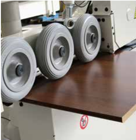
Device for the automatic insertion of the panels coming from the handling system placed at the entrance of the machine (opt).
