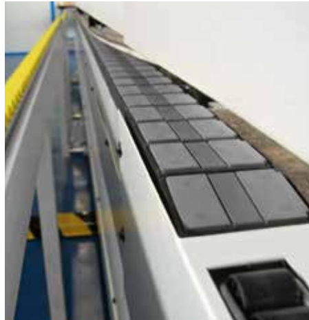
Panel feed track with pads with specific design, high stability and gentle grip.
