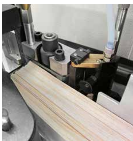
Application of edging in ready-cut strips, veneer or rigid plastic (unicolor, formica, PC).
