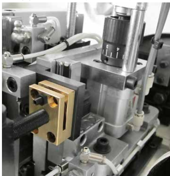
Automatic vertical double position by HMI for the trimming of plastic or wood edging (std). Manual micro-adjustment of the stop.
