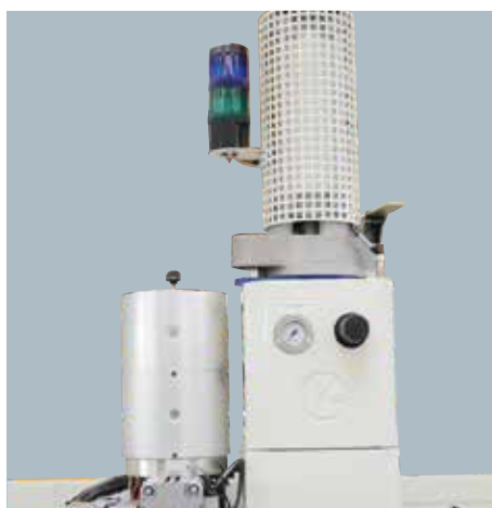
Quick changeover of the glue type, from EVA to PU or vice versa, with manual selection of the pre-melter.
