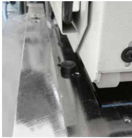
Productivity optimized thanks to the panel spacing device (std) which determines the best distance between panels according to the various conditions.
