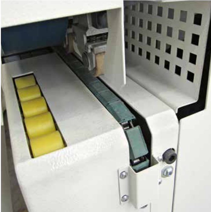
Outfeed transfer for the machine integration with external automation systems (opt).
