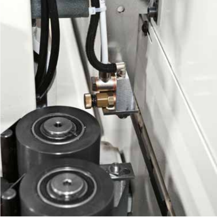
Liquid to cool the temperature of the glue in the area exceeding the edge, after the edging, in order to keep the tools clean for the subsequent processing.
