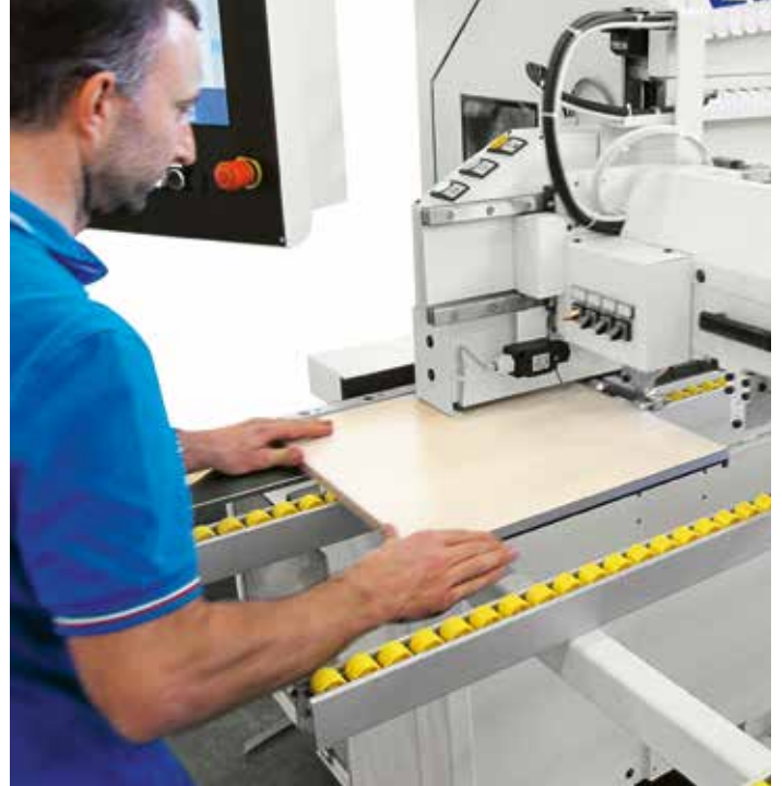
Easy Order M manual infeed device for easy and error-free introduction of panels orthogonally to the feed direction. For dimensions up to 2,200 mm x 1,200 mm (opt).
