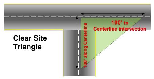
obstructions as measured between the height of three feet (3') up to ten feet (10') above the surface of the street. A one-hundred-foot clear sight triangle shall be maintained at all street intersections.
