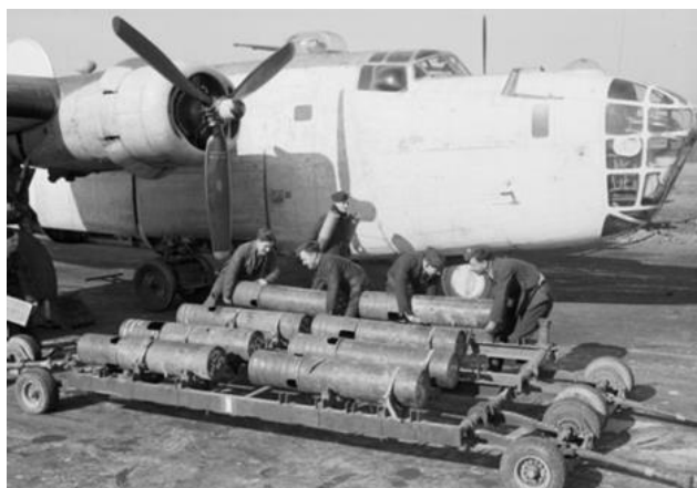
Figure 4 Armourers unload 250lb depth charges from a bomb trolley and load onto a Consolidated Liberator GR Mk VA of No 53 Squadron RAF at St Eval 1944
