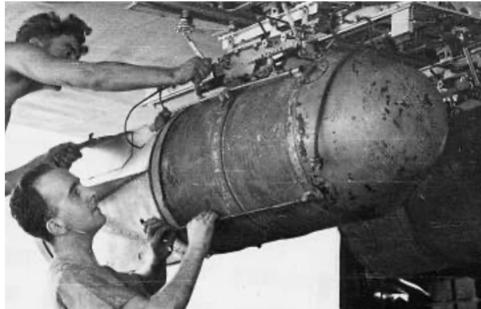
Figure 12 A MKVII depth charge being armed on a Sunderland bomber.
