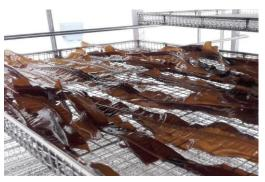
Our seaweed is dried within chambers containing dehumidifiers and fans to maintain strong airflow around the chamber. At the end of the cycle, the temperature is raised to around 40- $45^{\circ}$ C. All our seaweed is dried to below a water activity (A<sub>w</sub>) of 0.60, below which microorganisms cannot proliferate. Indeed, typically our seaweed is down to 0.30-0.45 A<sub>w</sub> when removed from the drying chambers.
