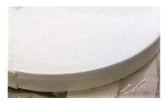
One such bespoke example has been a ribbon developed with binder seeding efficiencies in mind. The fluffy surface, and high surface area to volume ratio ensures the maximum amount of binder could remain fixed to the line per metre without increasing the overal amount of material as much as rope would. This ribbon has been used for binder deployments in Europe in place of ropes. We saw this as
