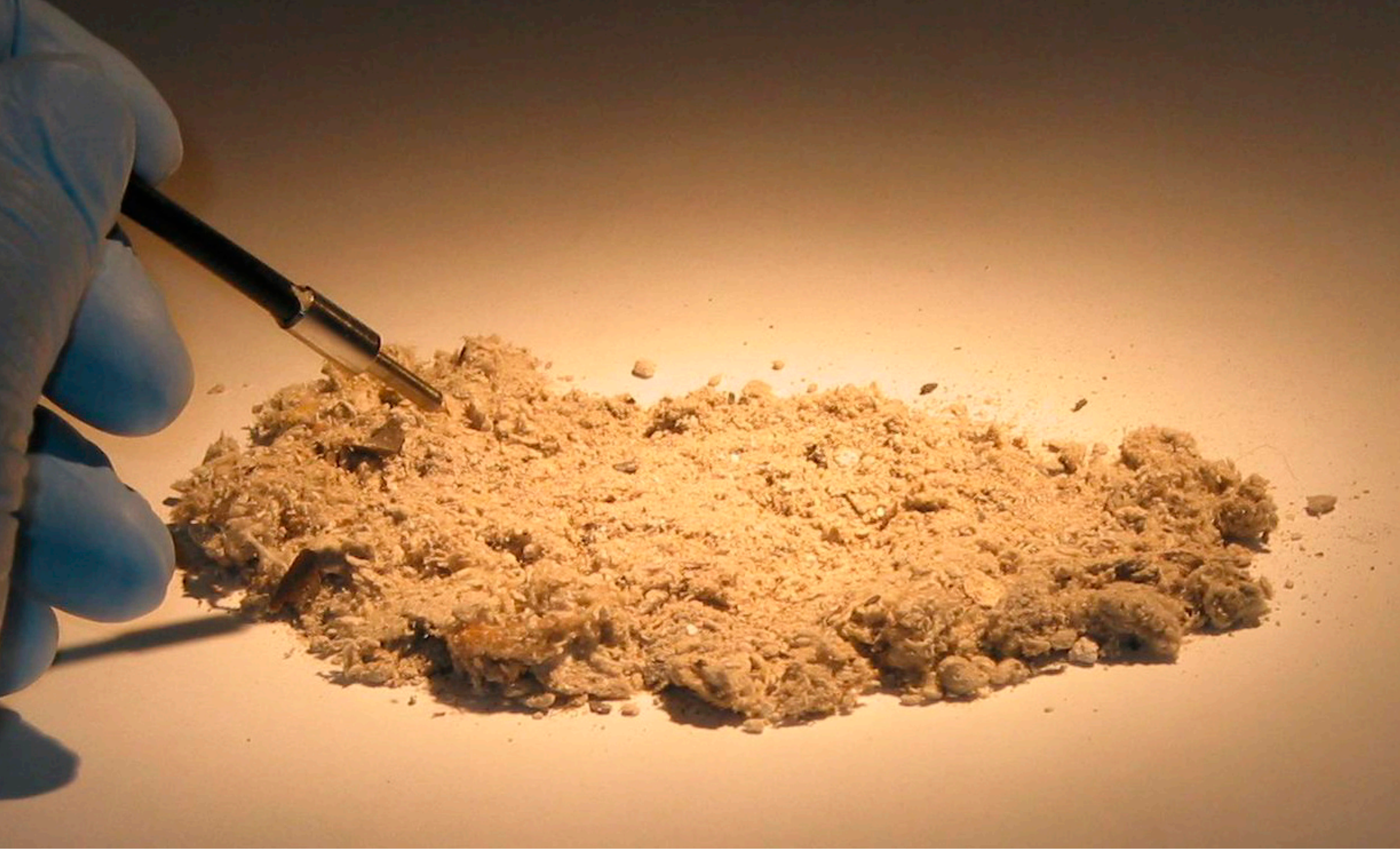
Closeup of sample WTC01-14 being measured with a spectrometer. The black cord with the steel tip is the fiber-optic probe of the spectrometer.
